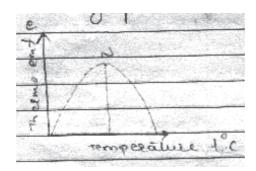
→ When temperature of reference junction is °c then the relation between thermo emt and temperature is obtained emprically as, are constants depending on the type of metals.
