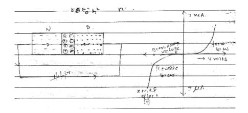
As shown in fig. the terminal of the battery is connected to P type & the -Ve terminal is connected to N-Type then such connection is called forward bais.
